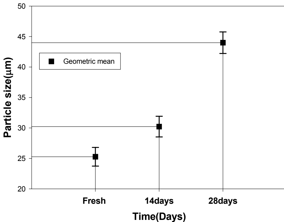
Figure 43. The geometric means and the geometric standard deviation of the particle size distribution of suspended metronidazole in freshly prepared sample of Formula A and after storage for 2 and 4 weeks at room temperature.
